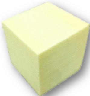
Low Density R-3.7 per inch Open-cell composition Soft, flexible foam Sponge-like texture
